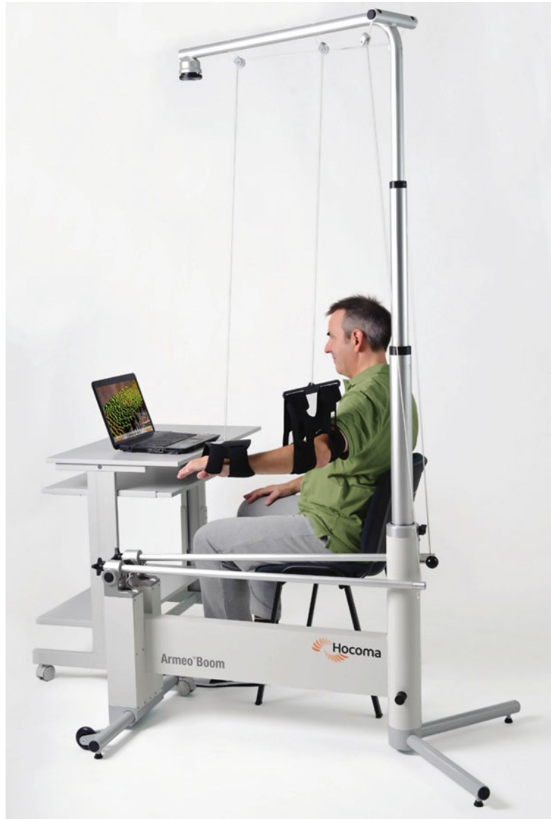
Fig. 23.2 The Armeo@Booom, a passive gravity support system
